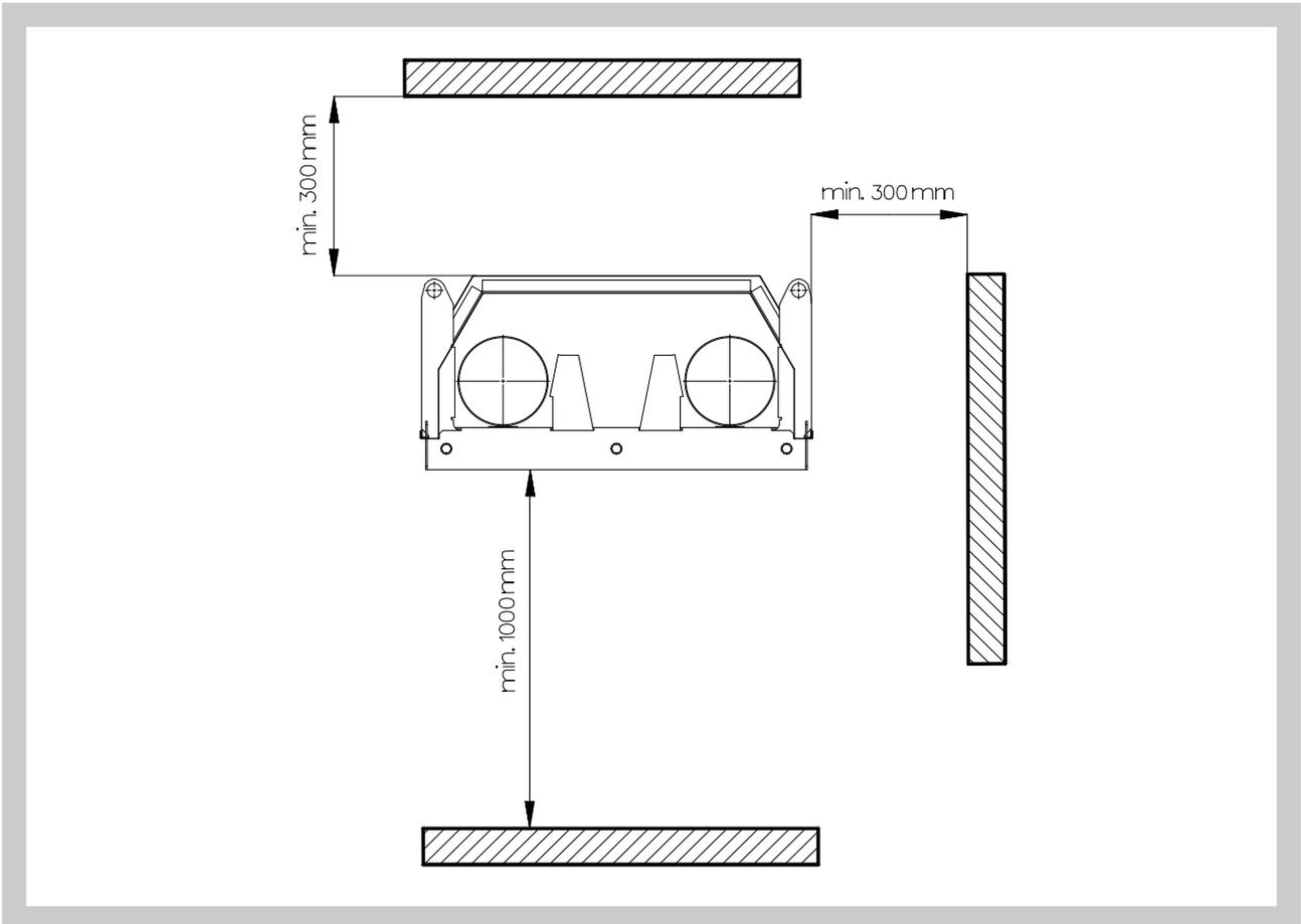
Fig. 6 Minimum safe distance of the infrared heater from walls and flammable objects
