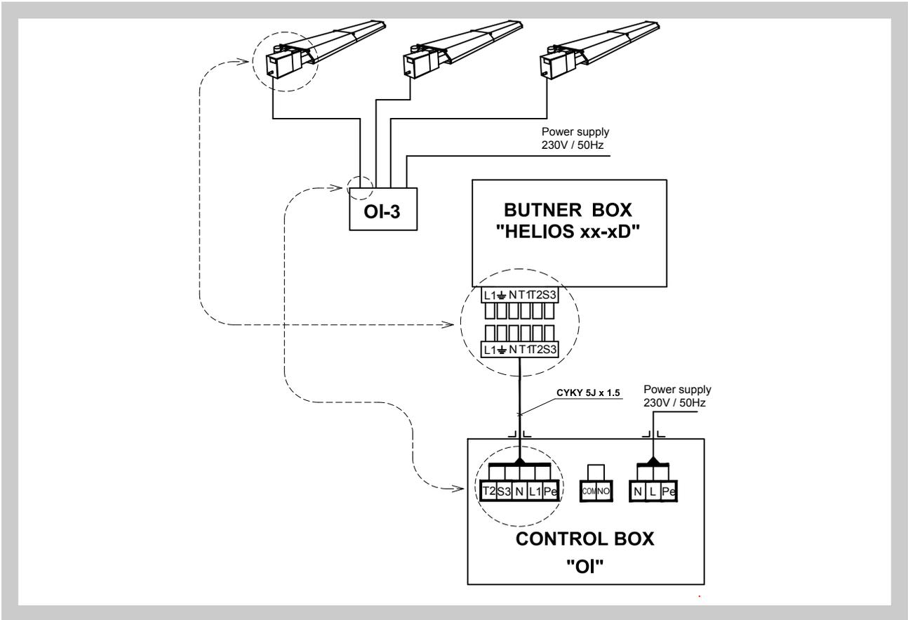
Fig. 16 Diagram of controlling the infrared heater HELIOS-S by control box OI D
