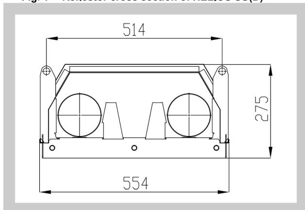
Fig. 2 Reflector cross section of HELIO SI(D)+
