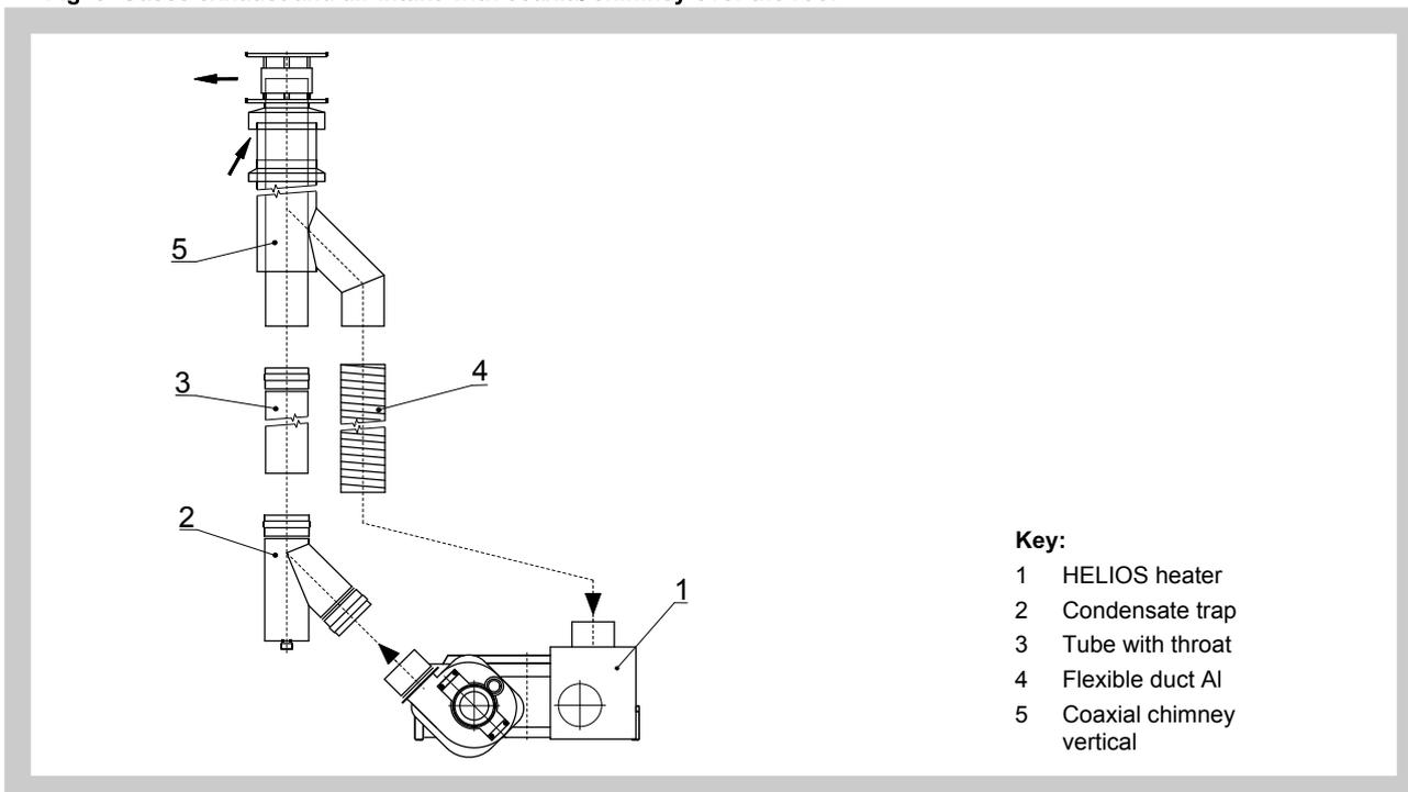
Fig. 9 Gases exhaust and air intake with separate ducts over the roof
