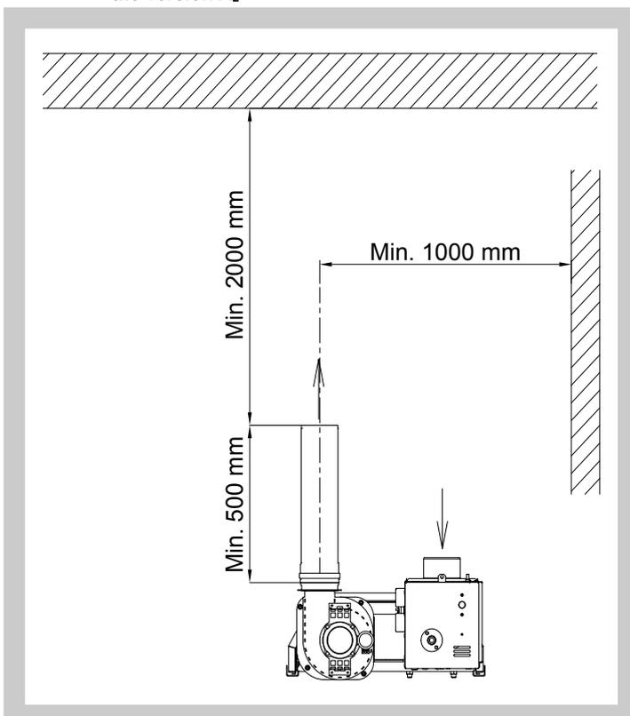
The flue gas exhaust is forced by the flue gas duct inside the building. The appliance is classified according to the flue into design version A<sub>2</sub>. The design and installation of the flue gas exhaust must comply according to the correct norm.
