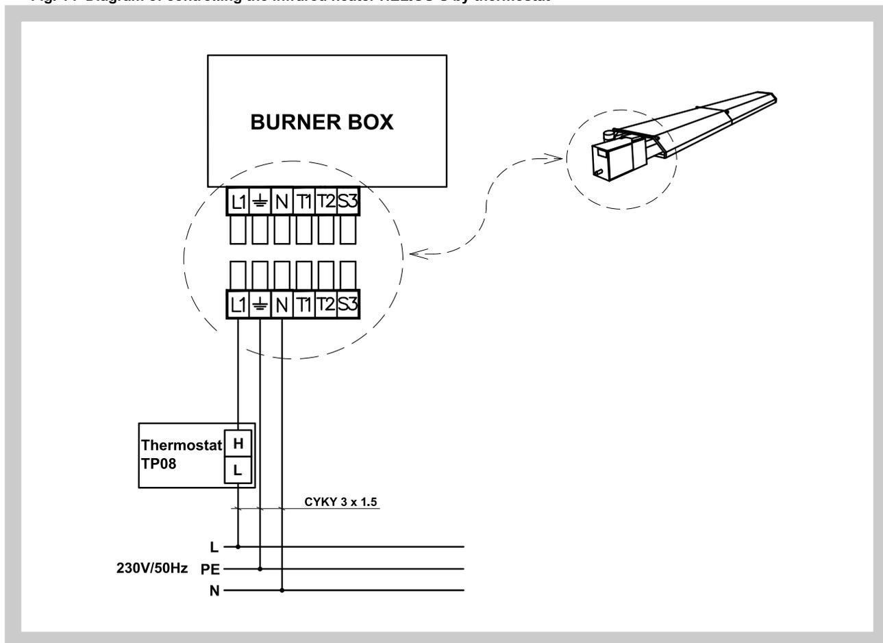
Fig. 15 Diagram of controlling the infrared heater HELIOS-S by control box OI
