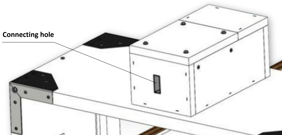
Example of pre-manufactured slot in the insulating box, with intumescent tape inside slot
