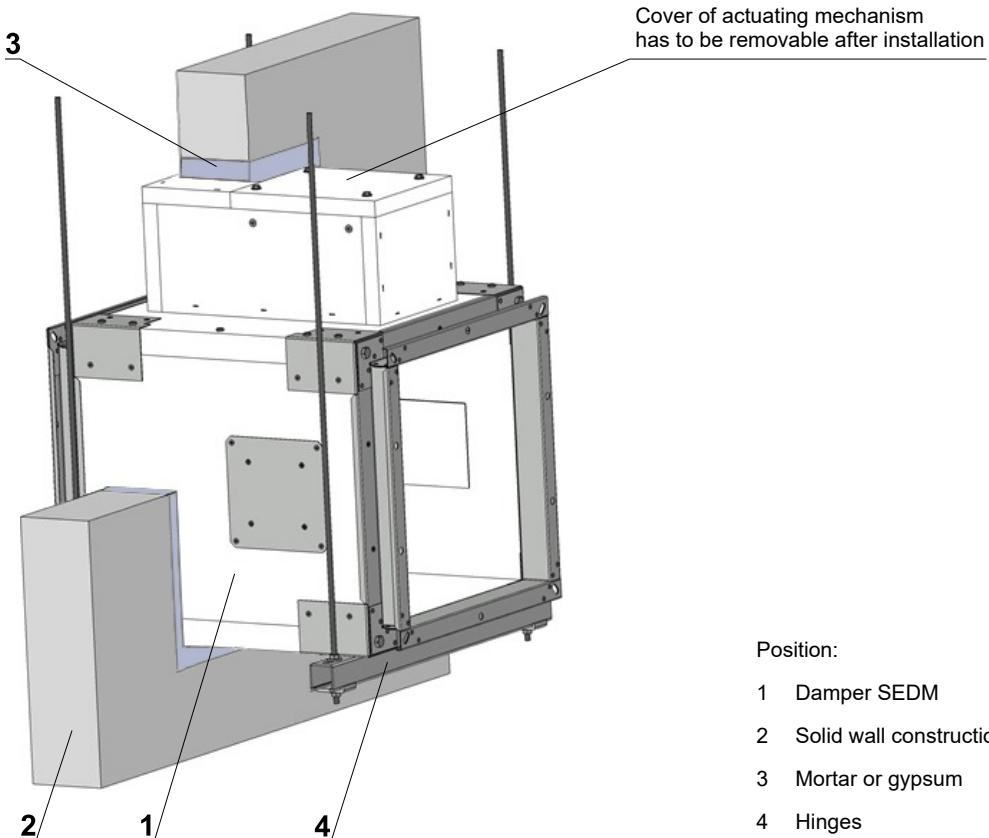
Fig. 24 Example of installation in solid wall construction of fire compartment - horizontal blade axis position.
