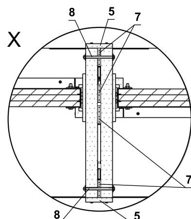
Fig. 45 2 dampers side by side - gypsum wall construction - Weichschott (Ablative Coated Batt)
