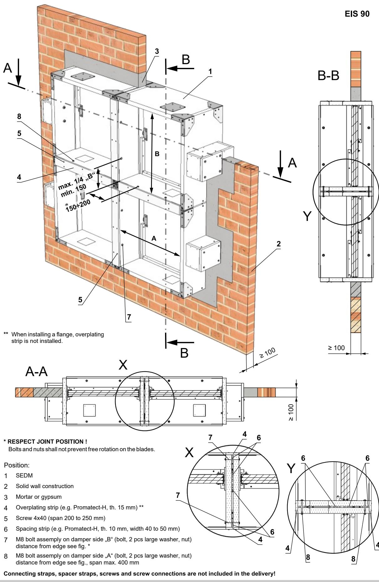
Fig. 50 4 dampers - solid wall construction - Weichschott (Ablative Coated Batt)
