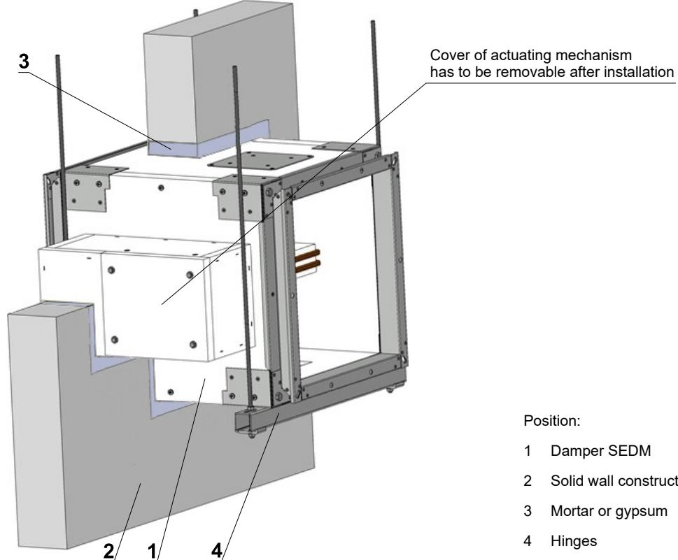
**Fig. 25 Example of installation in solid wall construction of fire compartment - vertical blade axis position.**
