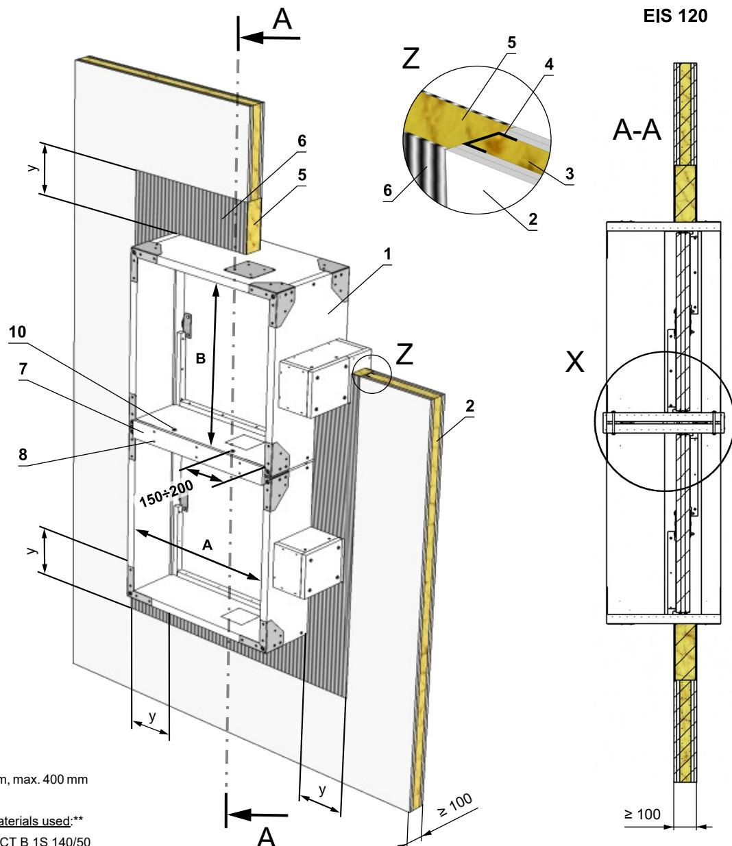
$y = \min, 30 \text{ mm}, \max, 400 \text{ mm}$
