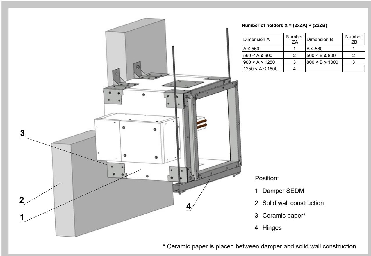
Fig. 39 Example of installation on solid ceiling construction of fire compartment - suspension.
