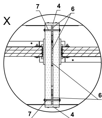
Fig. 44 2 dampers side by side - solid wall construction - Weichschott (Ablative Coated Batt)
