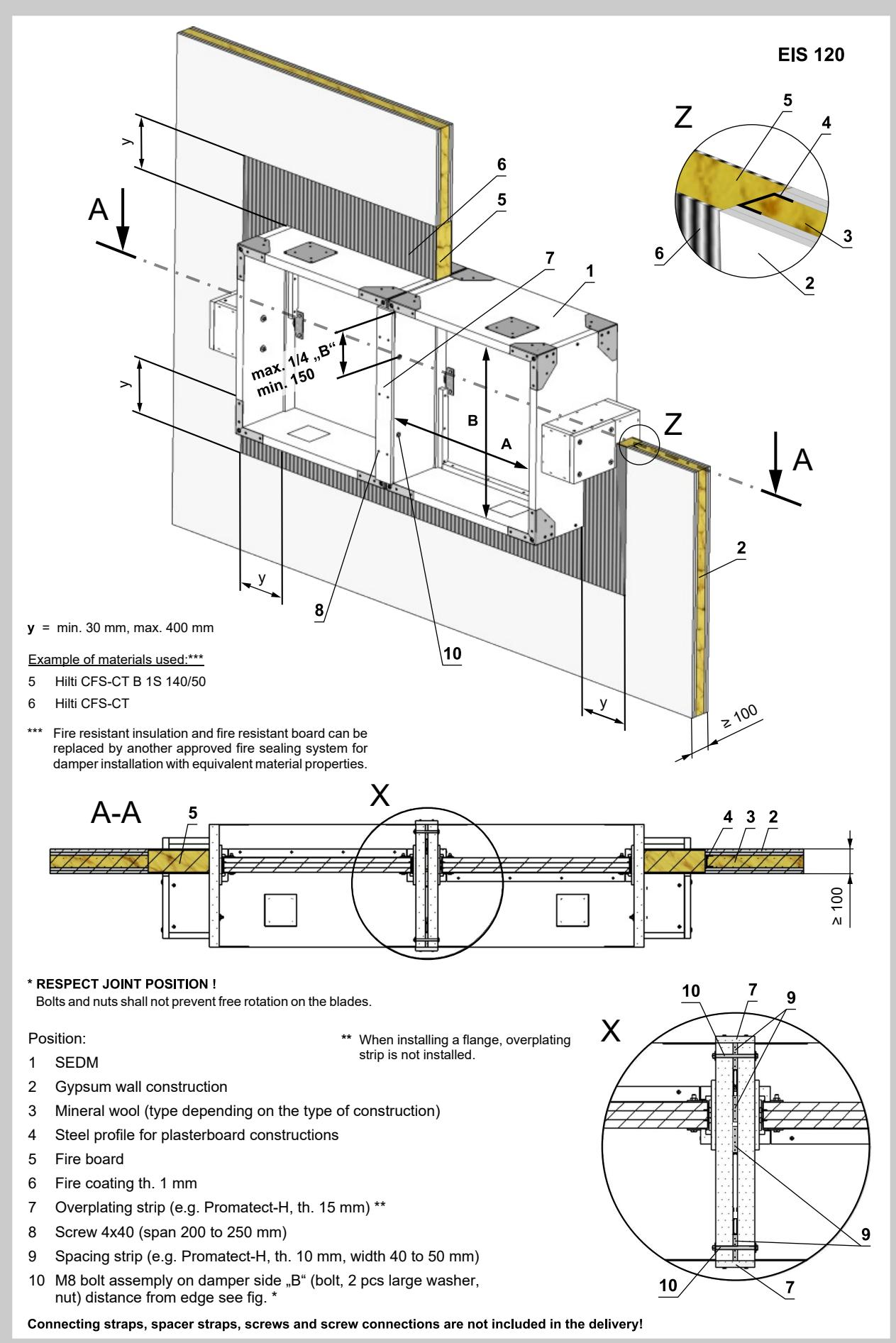
Fig. 46 2 dampers on top of each other - solid wall construction - mortar or gypsum
