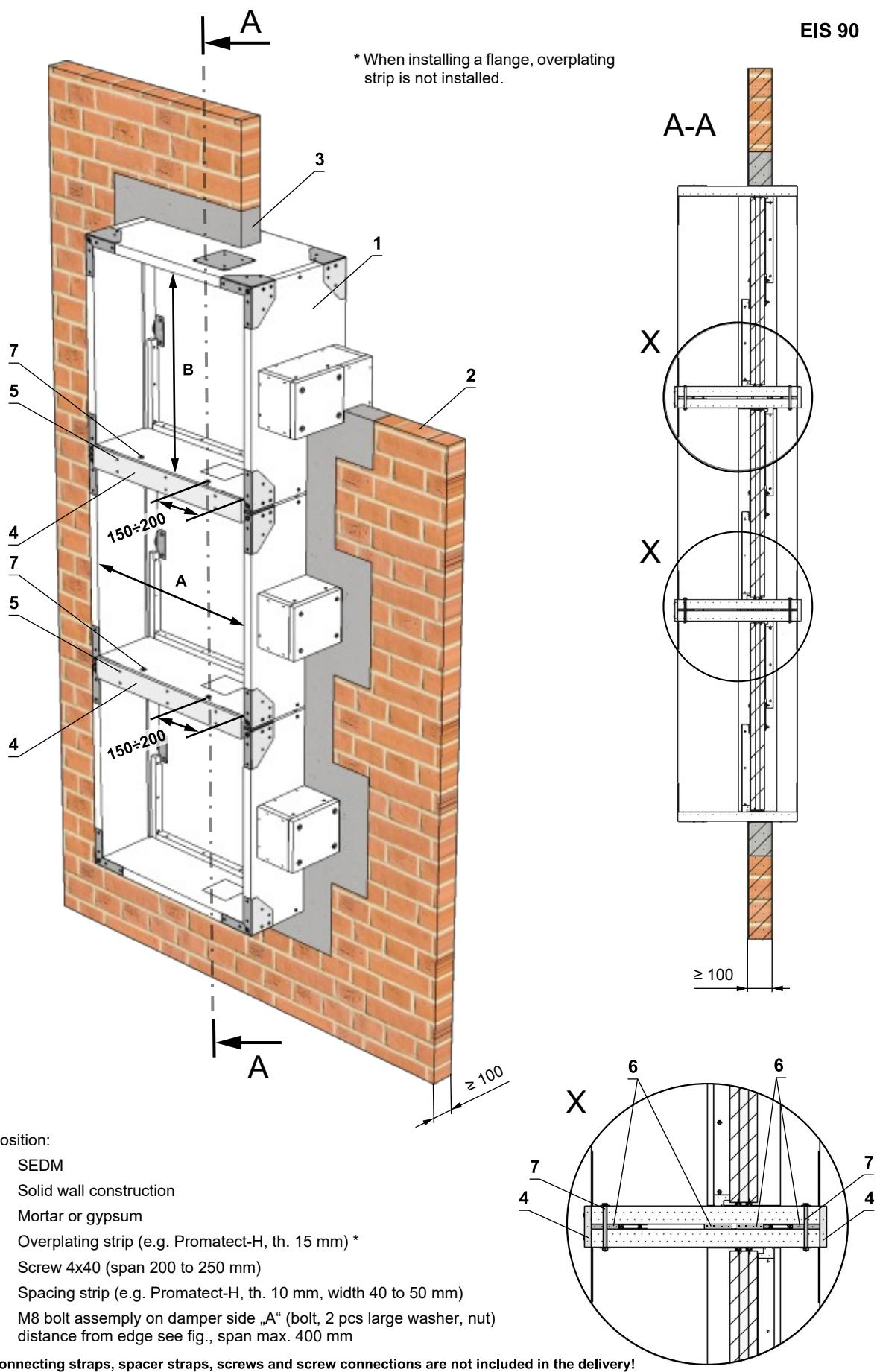
Fig. 53 3 dampers on top of each other - solid wall construction - Weichschott (Ablative Coated Batt)
