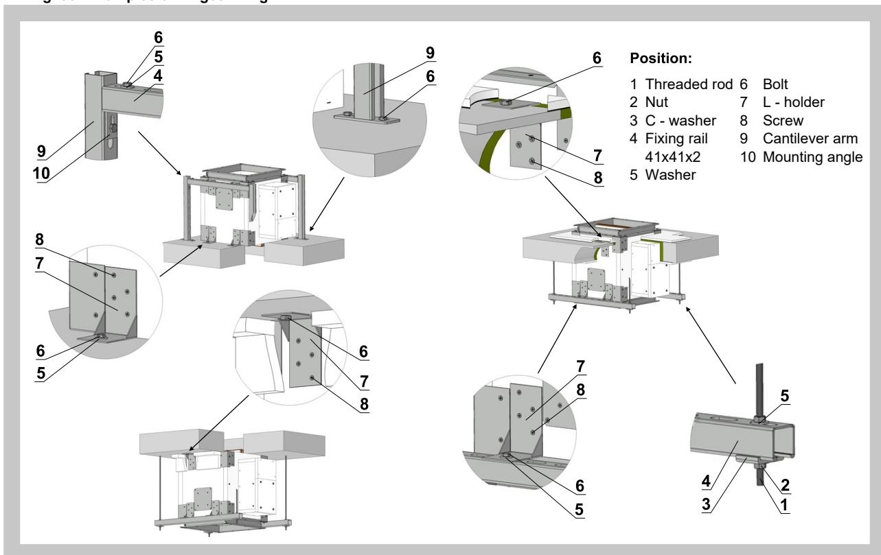
Fig. 57 Examples of damper connection to the duct
