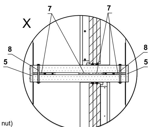
Fig. 54 3 dampers on top of each other - gypsum wall construction - Weichschott (Ablative Coated Batt)
