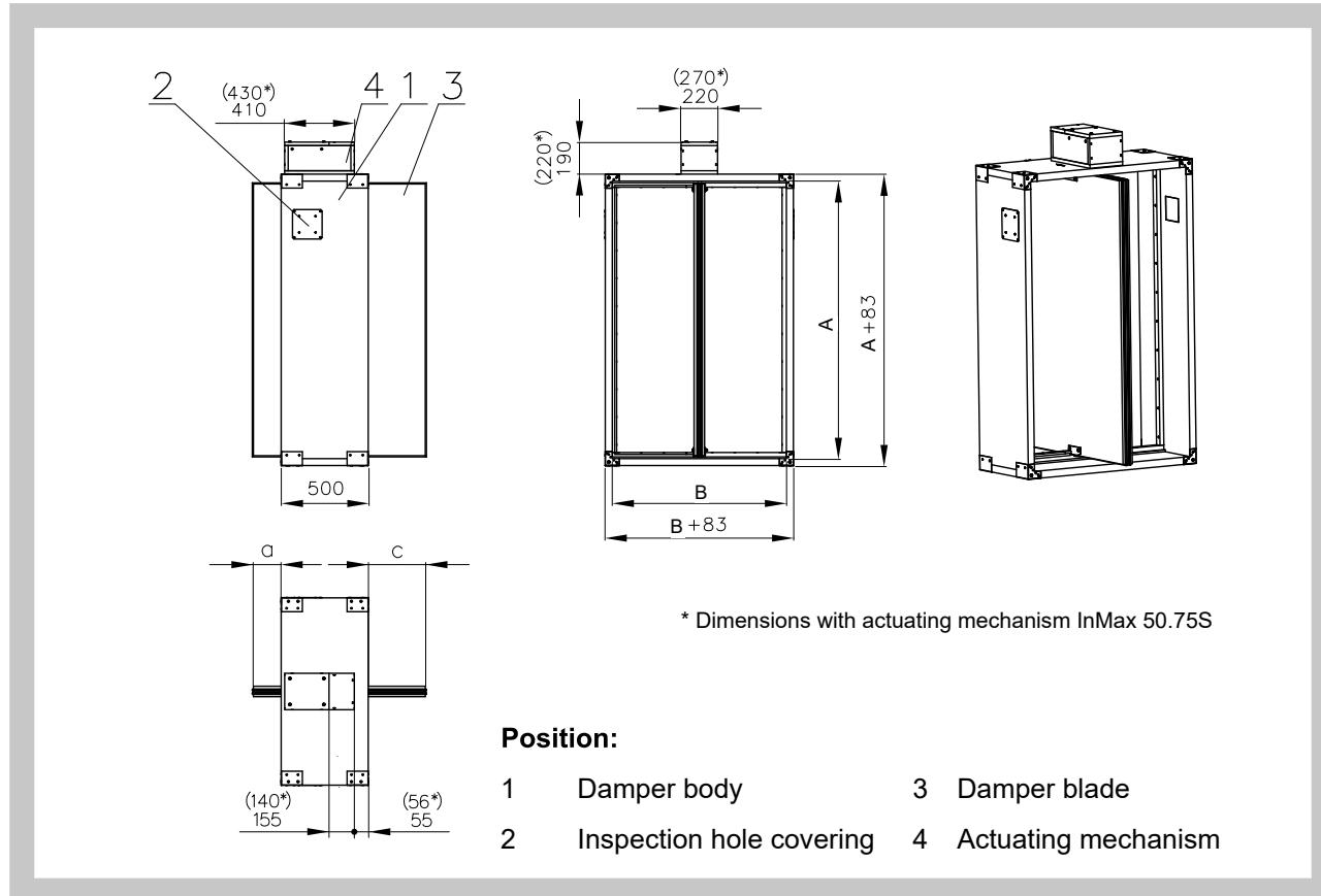
Fig. 16 Multi compartment smoke control damper with flanges
