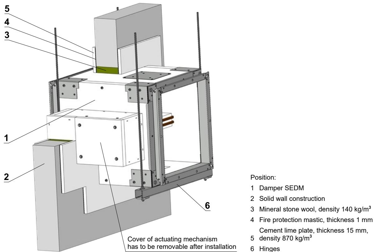
Fig. 23 Example of installation in solid wall construction of fire compartment - vertical blade axis position.
