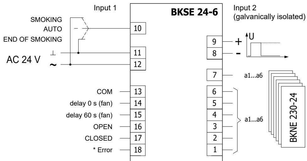
\* reverse output: fault = contact open
