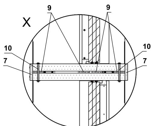
Fig. 49 4 dampers - solid wall construction - mortar or gypsum
