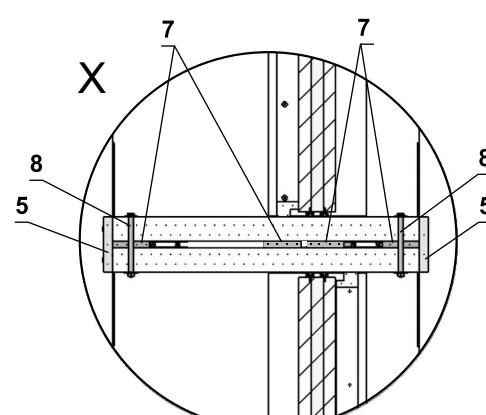
**Fig. 48** 2 dampers on top of each other - gypsum wall construction - Weichschott (Ablative Coated Batt)
