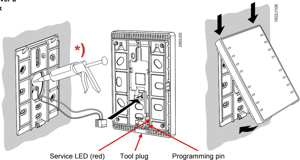
**\*)** The installing tube must be sealed or cold or warm air may enter the device and cause faulty temperature readings by the internal sensor.
