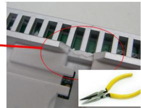
Remove the breakout on the housing before putting the cable into the gaining channel.
