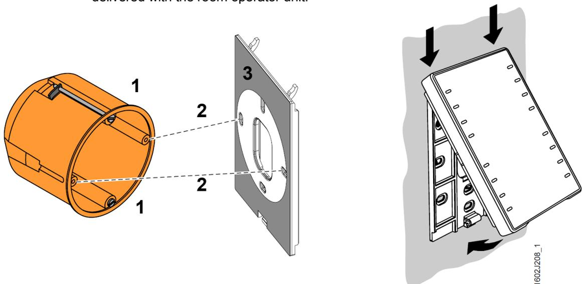
*The installing tube must be sealed or cold or warm air may enter the device and cause faulty temperature readings by the internal sensor.*
