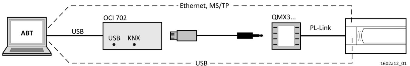
Connect the ABT to load the application in the room automation station, or for service purposes:
