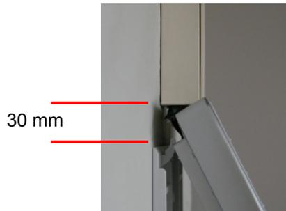
Keep a distance of 30 mm (from above) / 20 mm (from below) to the base plate, so that the device can be snapped onto the base plate.
