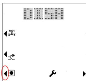
Press "Fact. Reset" (Key 4). The device is locked and reboots within 10 seconds. The room automation station deletes it from its device list. During this time, it is safe to remove the device from the network.
