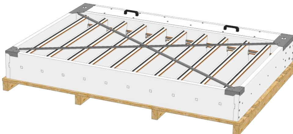
2. Place handling inserts between the top blade and the damper housing.
