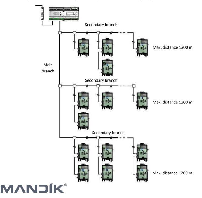
BKS64-PL is control and indication device for motorized fire dampers that can control
