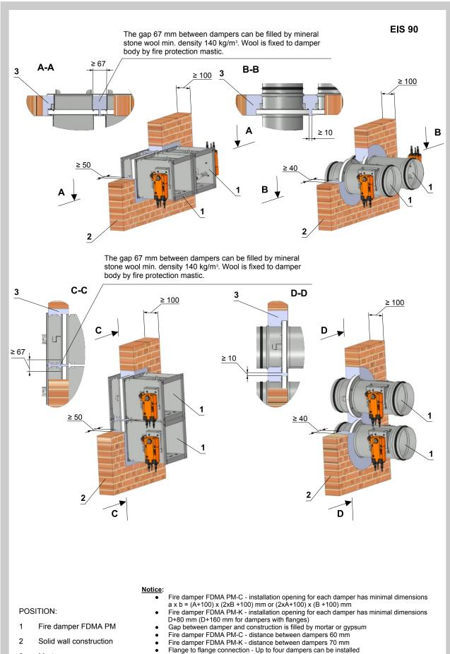
Fig. 41 Solid wall construction - flange to flange - mortar or gypsum
