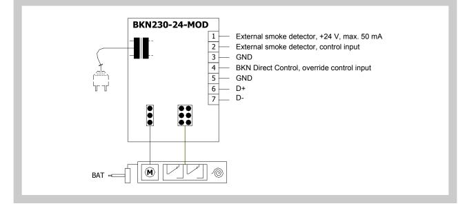
Fig. 23 Design with communication and supply device BKN 230-24-MOD, with actuating mechanism BF 24-TN-ST (BFL 24-T-ST, BFN 24-T-ST) and smoke detector ORS 142 K
