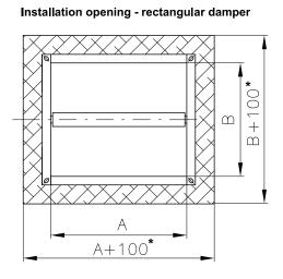
\* The recommended dimension of the installation opening is from 25 mm to 50 mm on the both sides (it means from A+50 to A+100 or B+50 to B+100)
