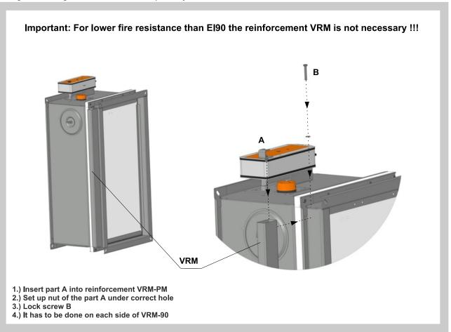
NOTICE: For dampers with A ≥ 800 and damper placement outside wall construction is necessary to use reinforcement VRM-PM.
