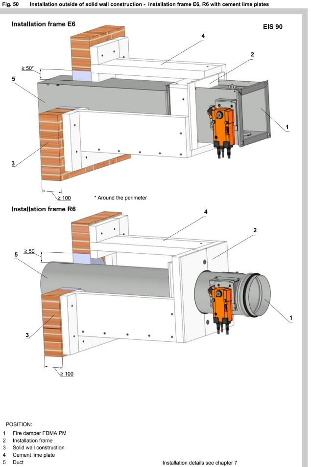
Installation outside of solid wall construction - installation frame E6, R6 with cement lime plates
