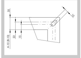
Fig. 35 Flage of rectangular damper - INSTALLATIONS SIDE
