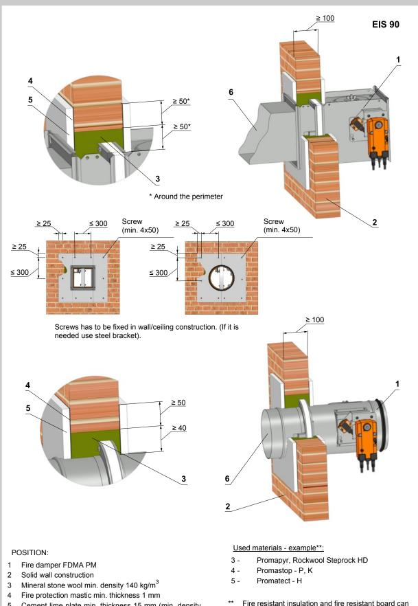
5 Cement lime plate min. thickness 15 mm (min. density 870 kg/m^3)
