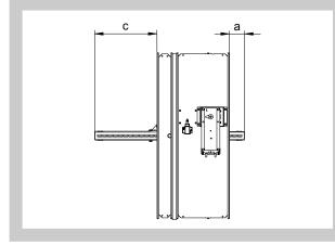
Fig. 33c Blade overlaps - round damper SPIRO
