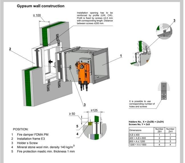
Notice: Gap between frame and solid (gypsum) wall construction must be filled by glue (PROMAT K84). Dampers has to be suspended in an appropriate manner see chapter 8.
