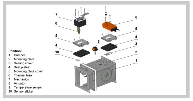
**2.2.** Design with actuating mechanism
