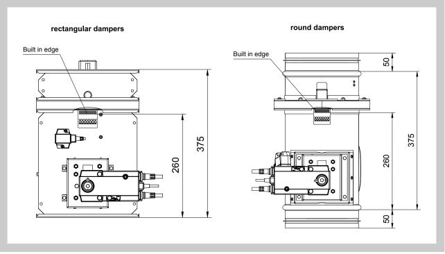
"Wall edge sticker" indicates the recommended edge of installation of fire damper into the fire partition structure (wall). The damper must be installed so that the entire damper blade - in the closed position - is located inside the fire separating structure (wall) and at the same time the control mechanism and inspection openings are freely accessible.
