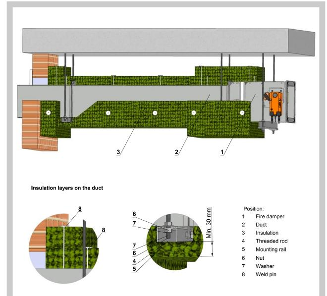
Fig. 103 Rectangular fire damper suspension on the wall - horizontal installation
