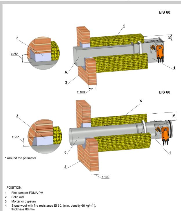
Fig. 96 Installation outside of solid wall construction - mineral wool - mortar or gypsum
