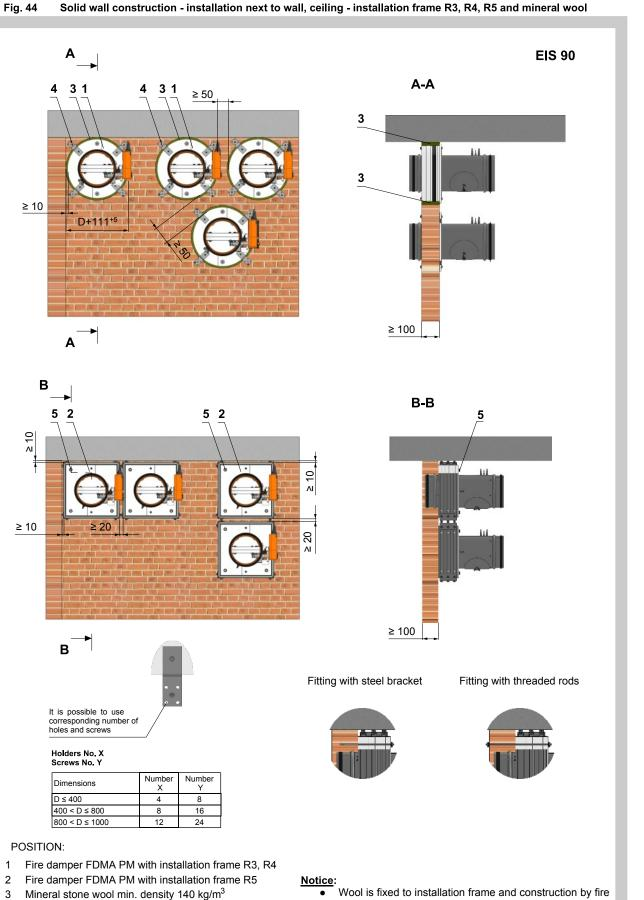
Solid wall construction - installation next to wall, ceiling - installation frame R3, R4, R5 and mineral wool
