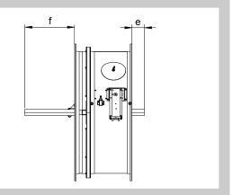
Fig. 33d Damper for SPIRO duct
