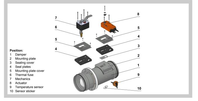
Fig. 10 Change of mechanical design for the motorised one or vice versa - RECTANGULAR
