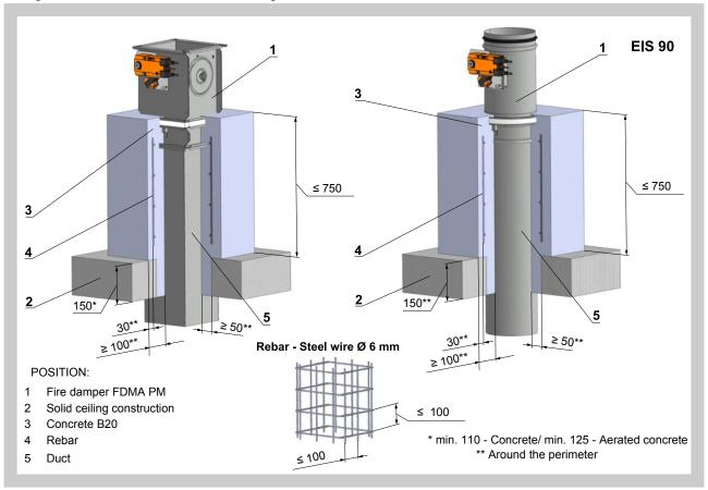
Fig. 59 Installation outside of solid ceiling construction - concrete and installation frame E4, R5
