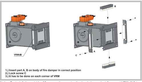
Notice: For installation outside of fire separating construction has to be used reinforcement VRM- III fixing.
