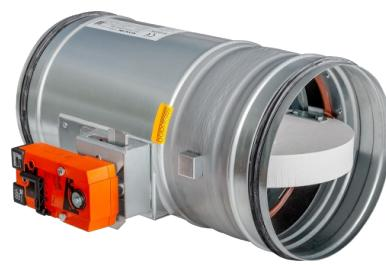
**1.1.** Multi compartment smoke control damper are shutters in the smoke exhaust duct systems. The dampers are designed to remove heat and combustible products (e.g. smoke) from effected fire compartments. In the event of fire the Smoke and Fire ventilation system opens the damper in the affected section and removes combustion products and heat from this section.
